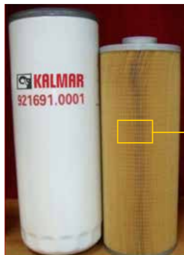
Fig. 1. Example of filter housing and filter element. Area of Fig. 2 shown with yellow square.
